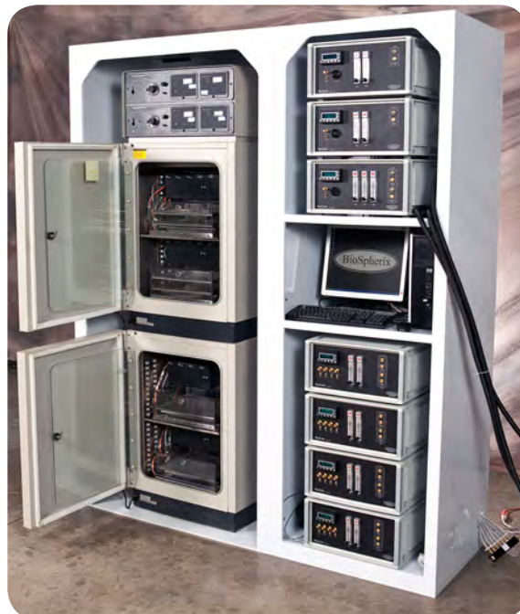
I-Hoods are normally designed for a single incubator with enough headspace to fit a GT series controller, but larger custom I-Hoods are available.
