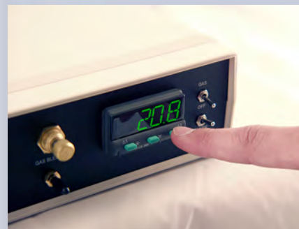
The ProOx 360 is easily operated through its front panel interface. Digital output displays current oxygen levels when not in use for programming.
